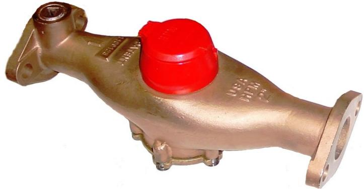
**INTRODUCTION:** ZENNER PERFORMANCE Residential Fire Meters utilize a unique patented multi-jet and dual element strainer to measure low flow rates comparable to traditional positive displacement meters with the high flows required of residential fire service meters. They are designed to measure cold and hot potable water where flow is in one direction only in residential and domestic use applications.
